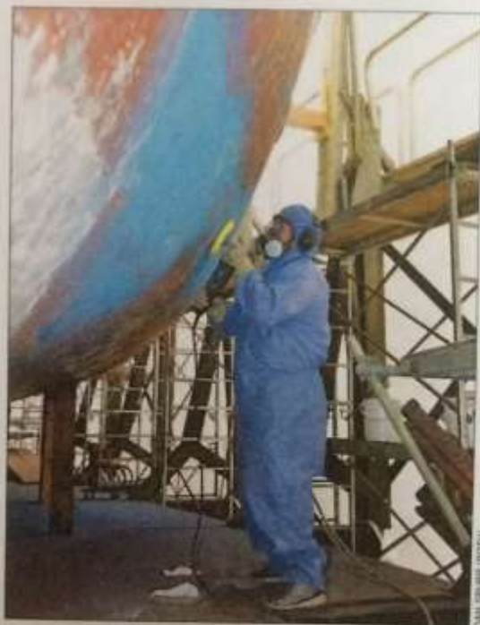
Above —Nearly all the vessel was enclosed in shrink-wrap before the anti-fouling paint could be stripped with spray-on DeFOUL and then hand-scraped. Right —The multi-coat Intersleek system required that the entire fiberglass hull be taken down to gelcoat and then sanded to a specific tooth profile.
