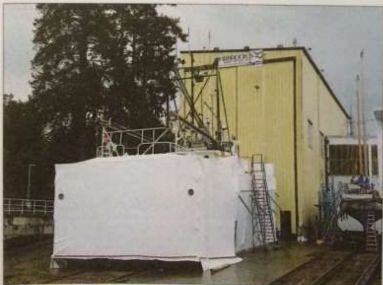
Above —Nearly all the vessel was enclosed in shrink-wrap before the anti-fouling paint could be stripped with spray-on DeFOUL and then hand-scraped. Right —The multi-coat Intersleek system required that the entire fiberglass hull be taken down to gelcoat and then sanded to a specific tooth profile.
